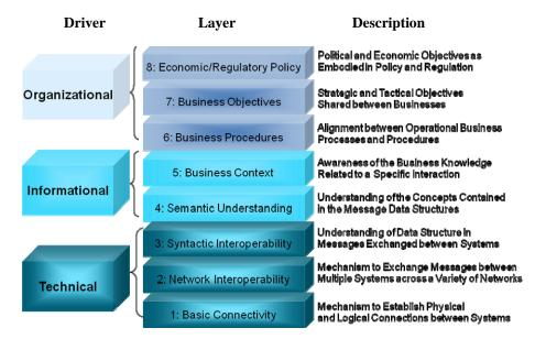
Figure 1. The GridWise Architecture Council's eight-layer stack provides a context for determining Smart Grid interoperability requirements and defining exchanges of information.
