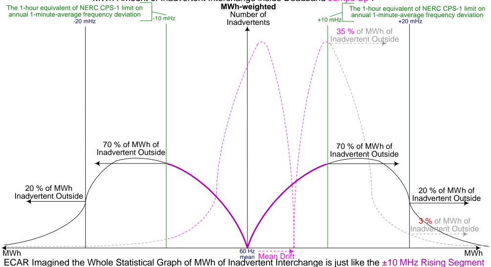
eCAR Imagined the Whole Statistical Graph of MWh of Inadvertent Interchange is just like the ±10 MHz Rising Segment of the Graph & Thought a Wide Deadband would Still Exclude Most of the Inadvertent MWh! The Opposite Happens: only 20 % of Total MWh of Inadvertent is outside a 20 mHz Bandwidth & Enough Frequency Drift Reduces that to 3 %!
